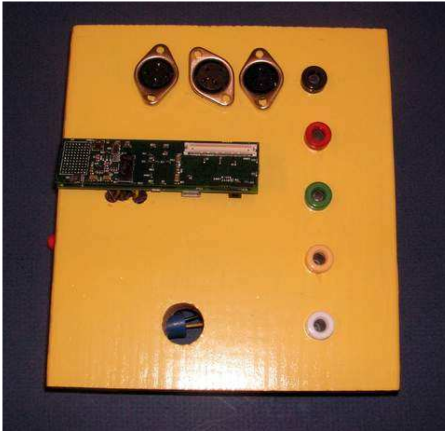
Figure 5.4: The mounting board for a single component. It contains three serial ports (along the top), 4 GPIO pins and a ground pin (along the right side), as well as a gumstix processor board mounted atop an expansion board.
